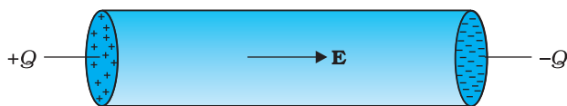
FIGURE 3.1 Charges +Q and -Q put at the ends of a metallic cylinder. The electrons will drift because of the electric field created to neutralise the charges. The current thus will stop after a while unless the charges +Q and -Q are continuously replenished.
