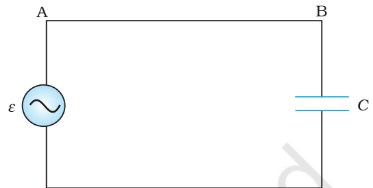
FIGURE 7.8 An ac source connected to a capacitor.
